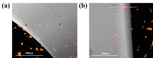
Figure 1. Phase contrast micrograph with DiI fluorescent image overlaid, demonstrating the cell morphology surrounding the (a) Co<sub>20</sub>Cr<sub>20</sub>Fe<sub>20</sub>Ni<sub>20</sub>Mn<sub>20</sub> and (b) SS 304 samples after 96 h of direct contact in cell culture. The metal samples are the black regions, cells are red.
